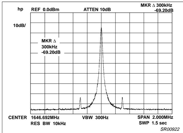
Figure 11. Fractional Spurs ( $f_{VCO} = 1646.7\text{MHz}$ ,  $NF = 1$ )
