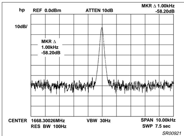
Figure 10. Close-In Phase Noise at 1668.3MHz
