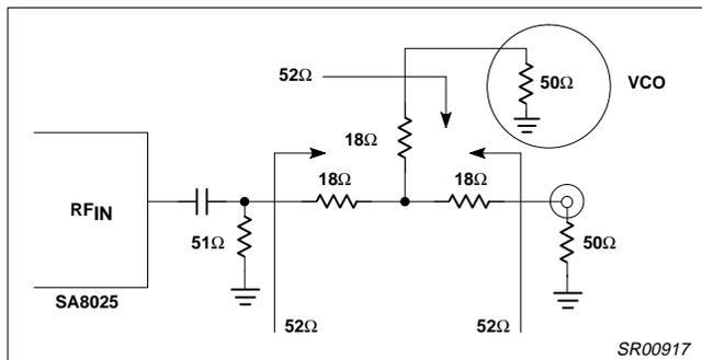
Figure 6. Matching Network for the RF<sub>IN</sub> Pin
