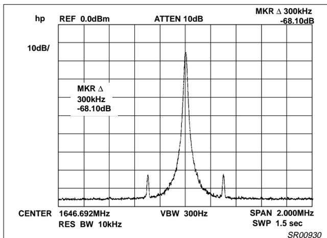
Figure 19. Fractional Spurs ( $f_{VCO} = 1646.7\text{MHz}$ ,  $NF = 2$ )
