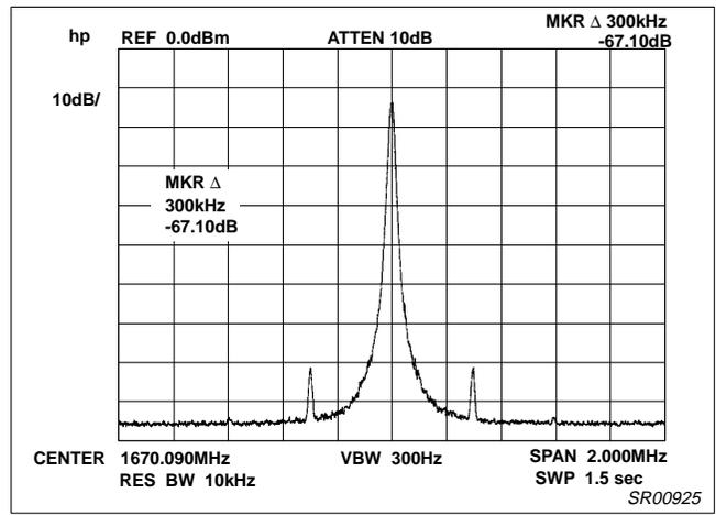
Figure 14. Fractional Spurs ( $f_{VCO} = 1670.1\text{MHz}$ ,  $NF = 7$ )
