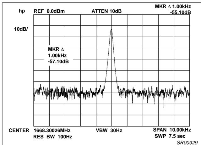
Figure 18. Close-In Phase Noise at 1668.3MHz
