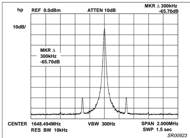
Figure 12. Fractional Spurs ( $f_{VCO} = 1648.5\text{MHz}$ ,  $NF = 7$ )
