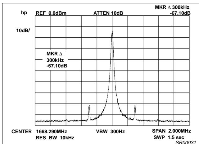
Figure 20. Fractional Spurs ( $f_{VCO} = 1668.3\text{MHz}$ ,  $NF = 2$ )
