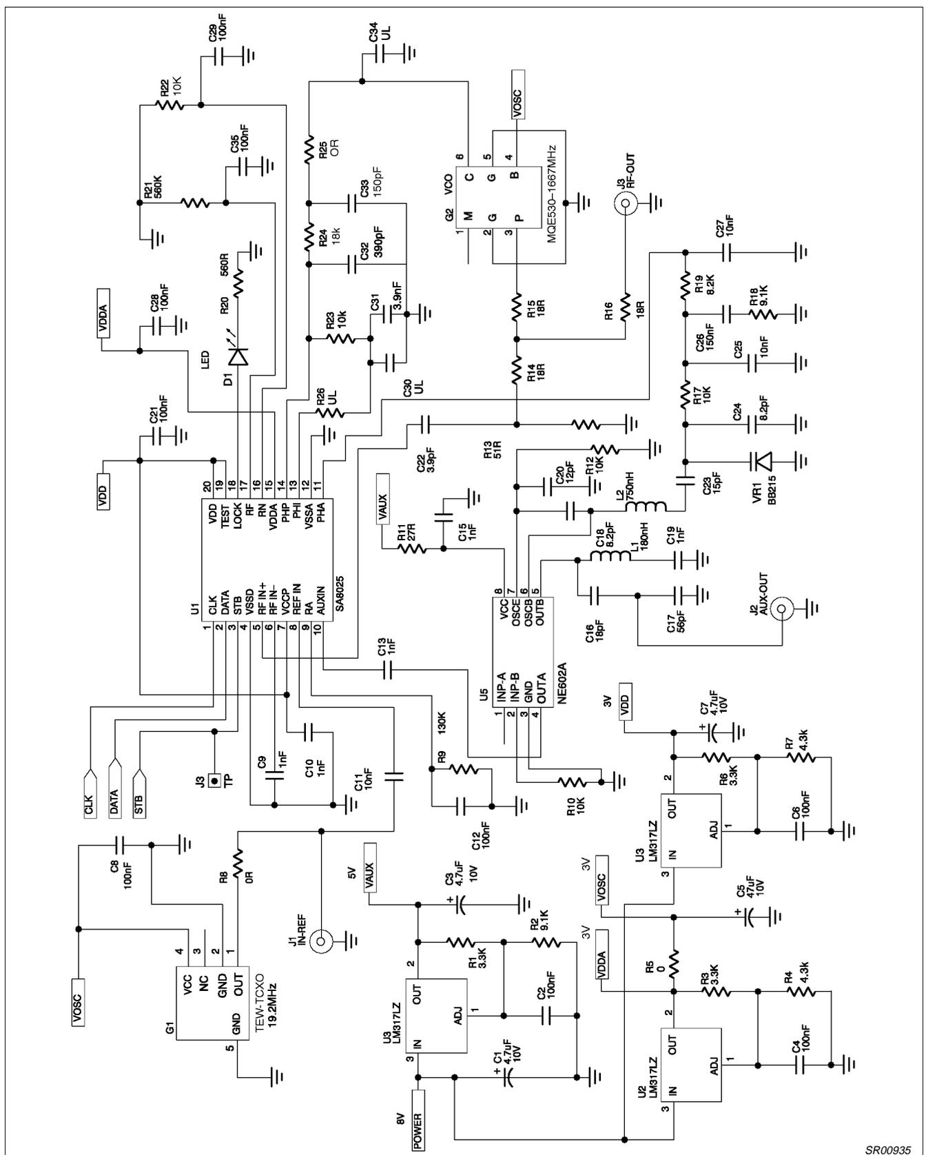
Figure 24. SA8025DK Application Circuit
