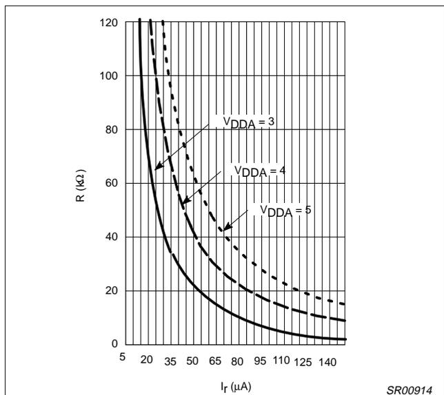
Figure 5. RN(RA) vs. I<sub>RN</sub>(I<sub>RA</sub>) for Different V<sub>DDA</sub>
