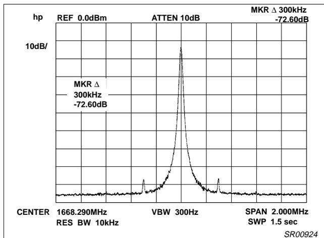
Figure 13. Fractional Spurs ( $f_{VCO} = 1668.3\text{MHz}$ ,  $NF = 1$ )
