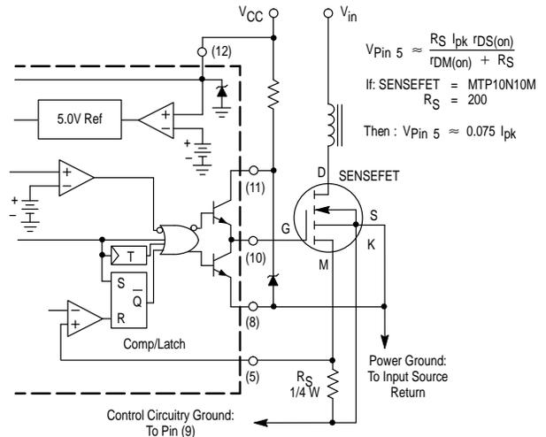
Virtually lossless current sensing can be achieved with the implementation of a SENSEFET power switch. For proper operation during over-current conditions, a reduction of the  $I_{pk(max)}$  clamp level must be implemented. Refer to Figures 19 and 21.
