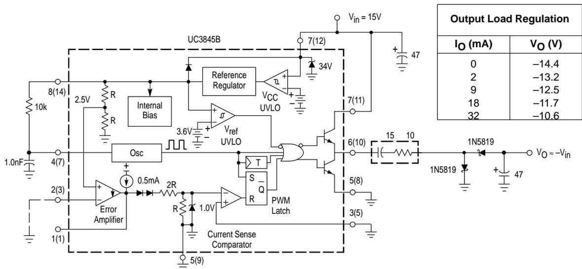
The capacitor's equivalent series resistance must limit the Drive Output current to 1.0 A. An additional series resistor may be required when using tantalum or other low ESR capacitors.
