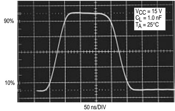
Figure 13. Output Cross Conduction
