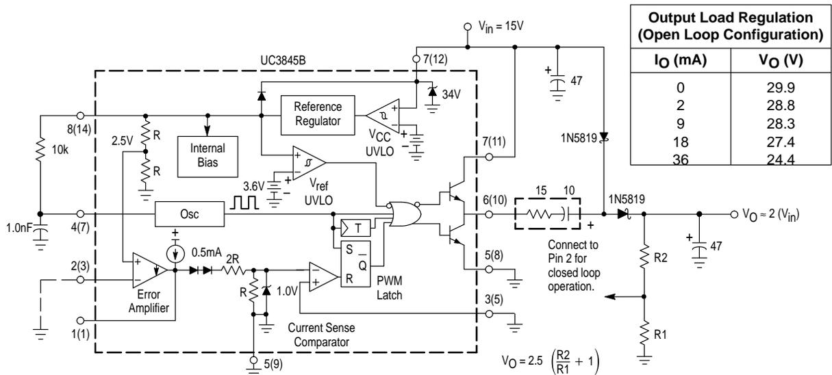
The capacitor's equivalent series resistance must limit the Drive Output current to 1.0 A. An additional series resistor may be required when using tantalum or other low ESR capacitors. The converter's output can provide excellent line and load regulation by connecting the R2/R1 resistor divider as shown.
