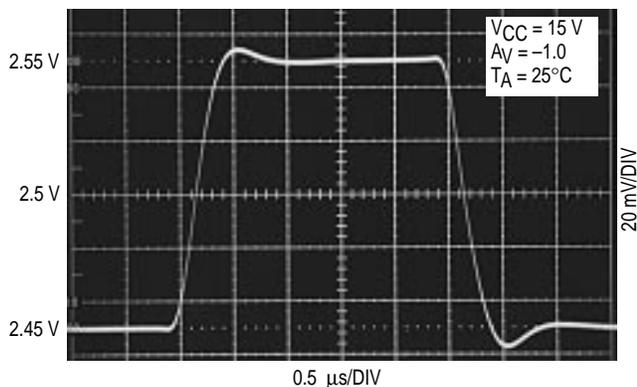
**Figure 4. Error Amp Large Signal Transient Response**
