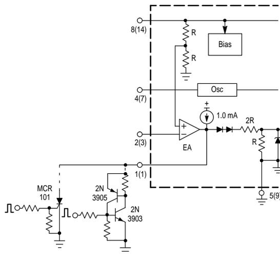
The MCR101 SCR must be selected for a holding of < 0.5 mA @ T<sub>A</sub>(min). The simple two transistor circuit can be used in place of the SCR as shown. All resistors are 10 k.
