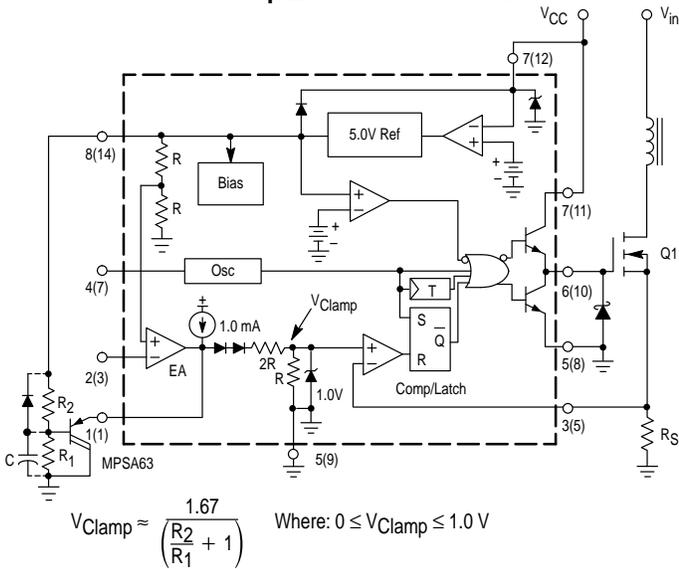
$$t_{Soft-Start} = - \ln \left[ 1 - \frac{V_C}{3V_{Clamp}} \right] C \frac{R_1 R_2}{R_1 + R_2} \quad I_{pk(max)} \approx \frac{V_{Clamp}}{R_S}$$
