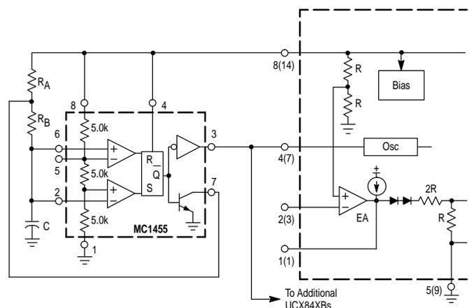
$$f = \frac{1.44}{(R_A + 2R_B)C} \quad D_{(max)} = \frac{R_A}{R_A + 2R_B}$$
