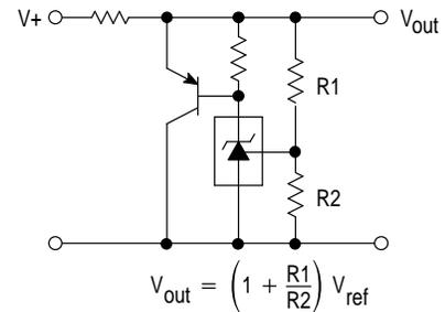
Figure 20. Output Control for a Three-Terminal Fixed Regulator
