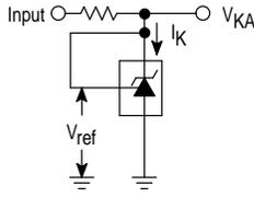
Figure 2. Test Circuit for  $V_{KA} > V_{ref}$
