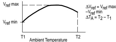
The average temperature coefficient of the reference input voltage, αV<sub>ref</sub> is defined as:
