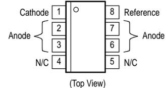
SOP-8 is an internally modified SO-8 package. Pins 2, 3, 6 and 7 are electrically common to the die attach flag. This internal lead frame modification decreases power dissipation capability when appropriately mounted on a printed circuit board. SOP-8 conforms to all external dimensions of the standard SO-8 package.
