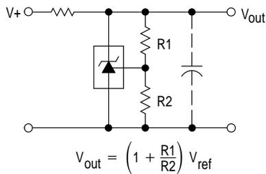
**Figure 19. High Current Shunt Regulator**
