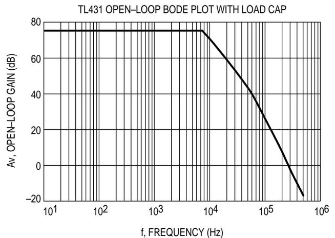
With three poles, this system is unstable. The only hope for stabilizing this circuit is to add a zero. However, that can only be done by adding a series resistance to the output capacitance, which will reduce its effectiveness as a noise filter. Therefore, practically, in reference voltage applications, the best solution appears to be to use a smaller value of capacitance in low noise applications or a very large value to provide noise filtering and a dominant pole rolloff of the system.
