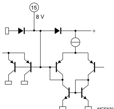
Fig.10 Pin 15: input equalizer switch.
