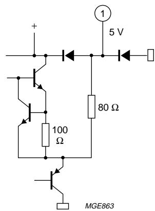
Fig.3 Pins 1 and 16: output channel.
