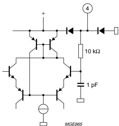
Fig.5 Pins 4 and 13: equalizer inputs.
