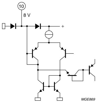
Fig.9 Pin 10: input head switch.
