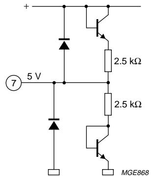
Fig.8 Pin 7: reference voltage.
