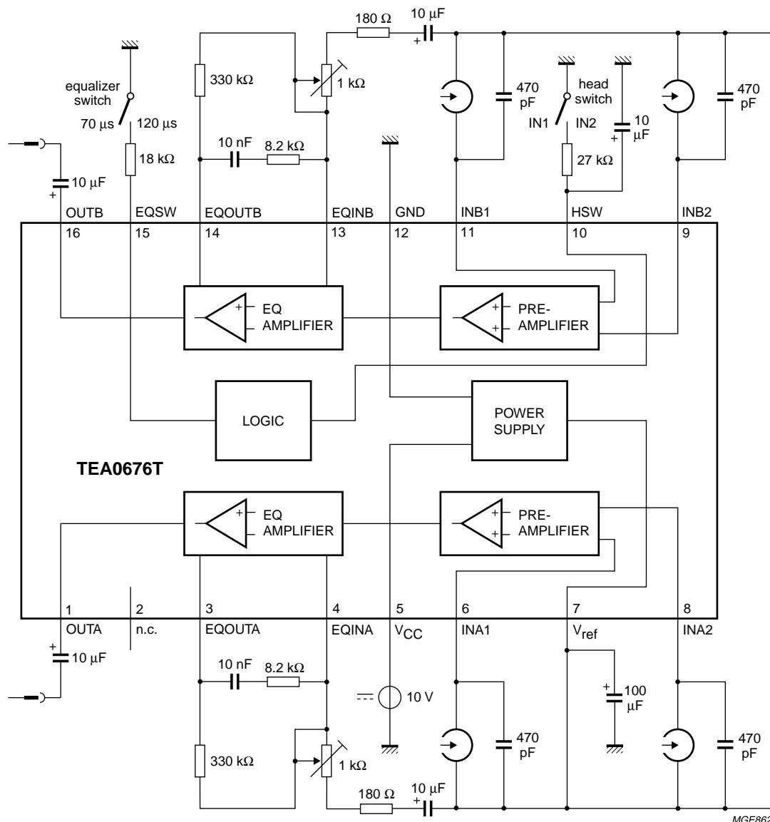
Fig.1 Block diagram.
