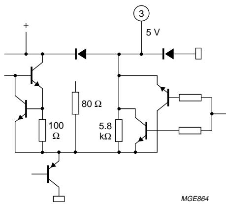
Fig.4 Pins 3 and 14: equalizer outputs.
