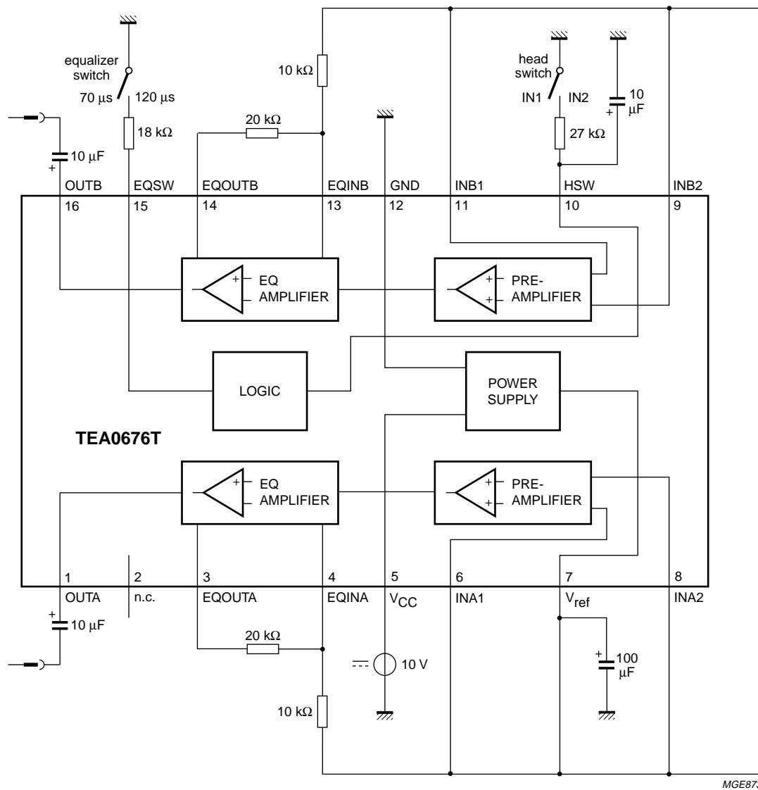
Fig.13 Noise test diagram.
