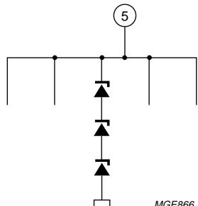
Fig.6 Pin 5: supply voltage.
