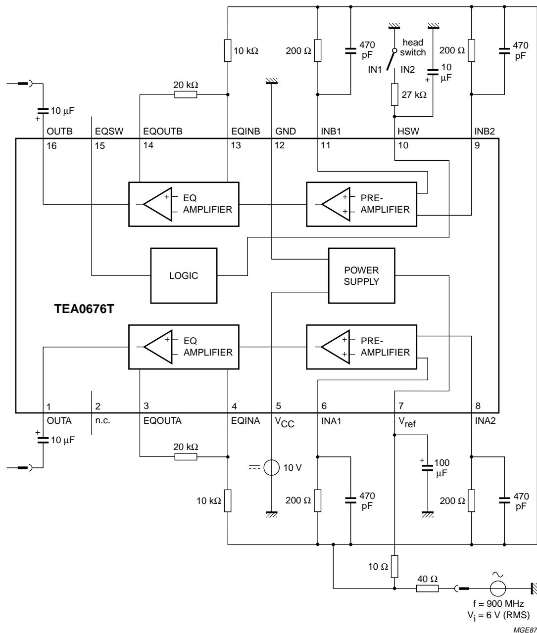
Fig.12 EMC test diagram.
