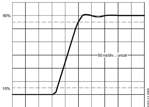
**Figure 3 : Rise Time**
