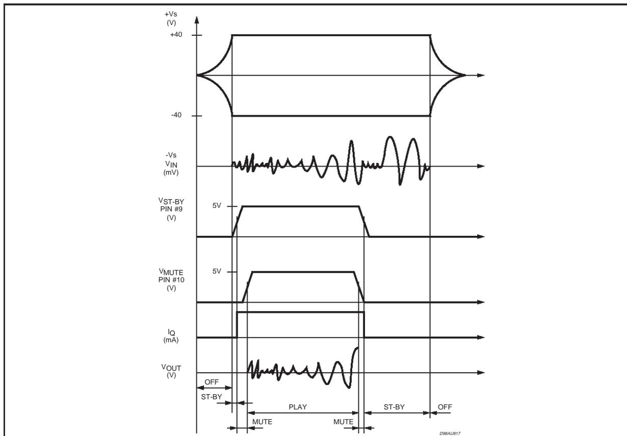
above, the device features a thermal shutdown circuit which initially puts the device into a muting state (@  $T_j = 150^\circ\text{C}$ ) and then into stand-by (@  $T_j = 160^\circ\text{C}$ ).
