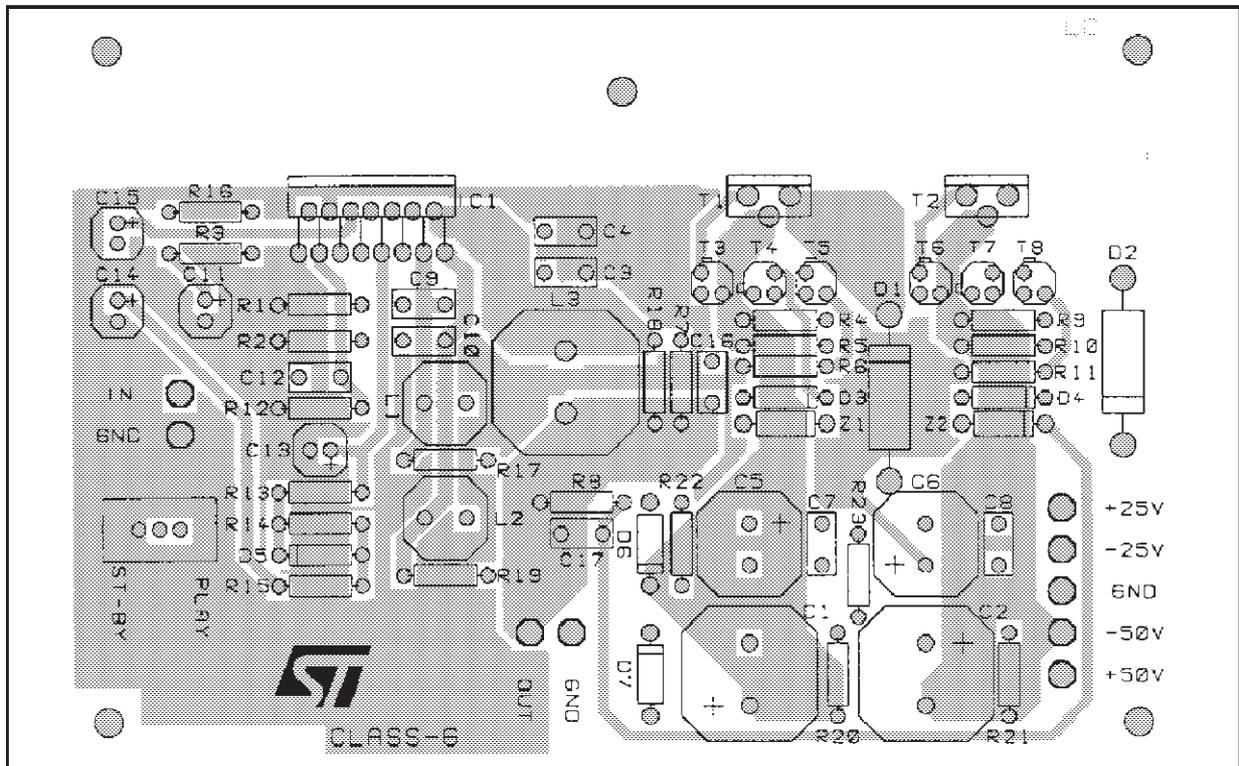
Figure 6b: PCB - Solder Side of the fig. 6.
