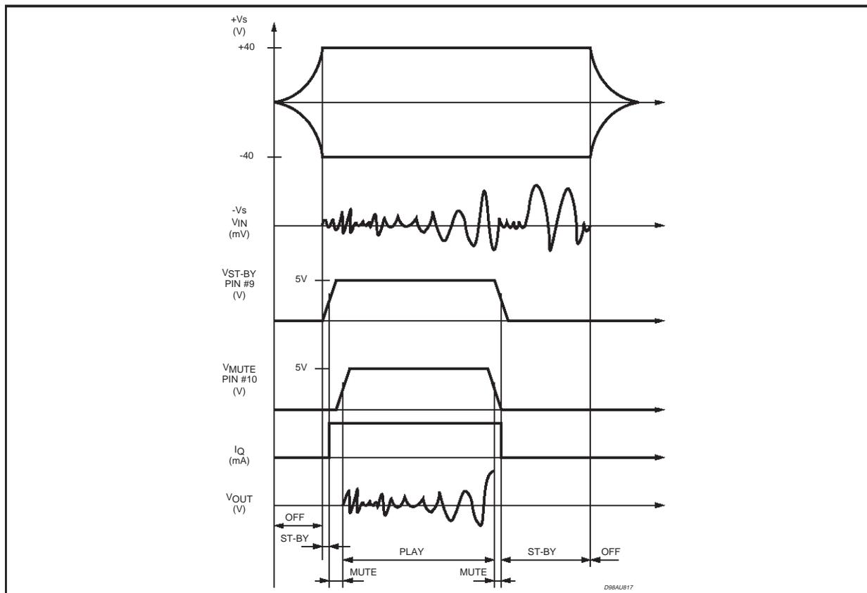
In addition to the overload protection described above, the device features a thermal shutdown circuit which initially puts the device into a muting state (@  $T_j = 150\text{ }^\circ\text{C}$ ) and then into stand-by (@  $T_j = 160\text{ }^\circ\text{C}$ ).
