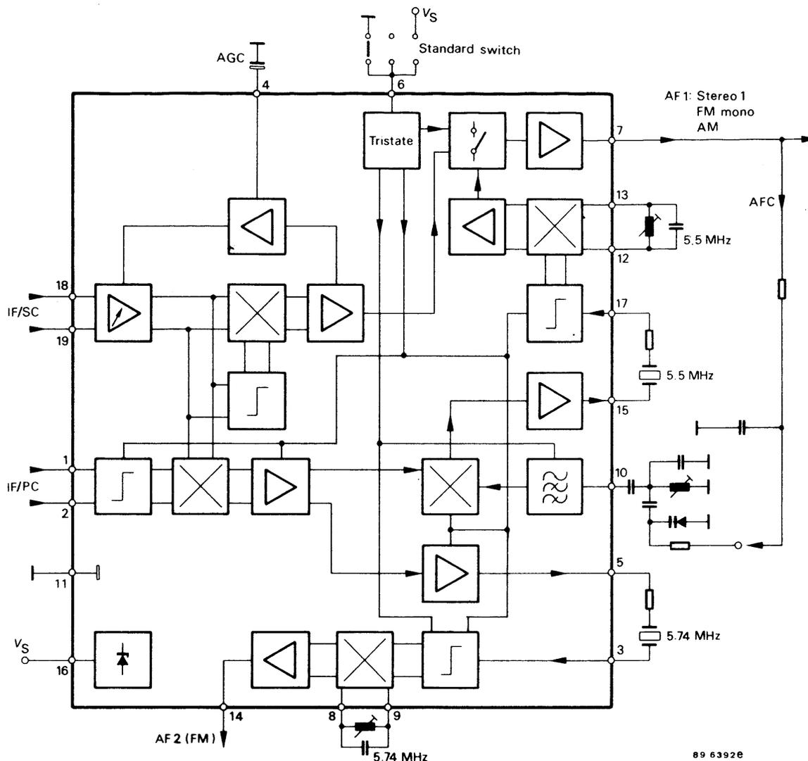
Figure 1 Block diagram
