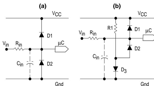
Figure 3 shows the clamping characteristics which are common to each of the six cells in the Peripheral Clamping Array.
