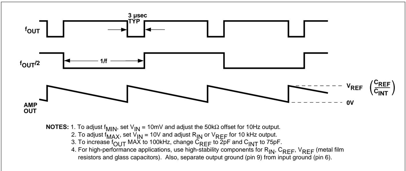
Figure 2 . Output Waveforms
