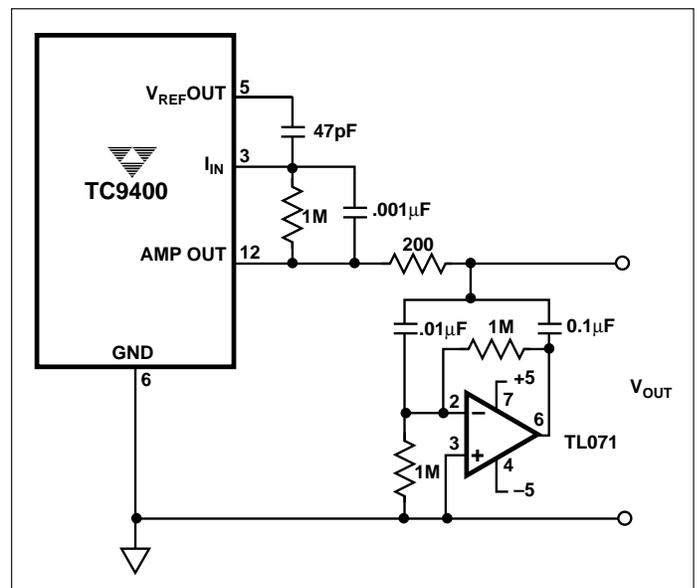
Figure 10. Ripple Filter
