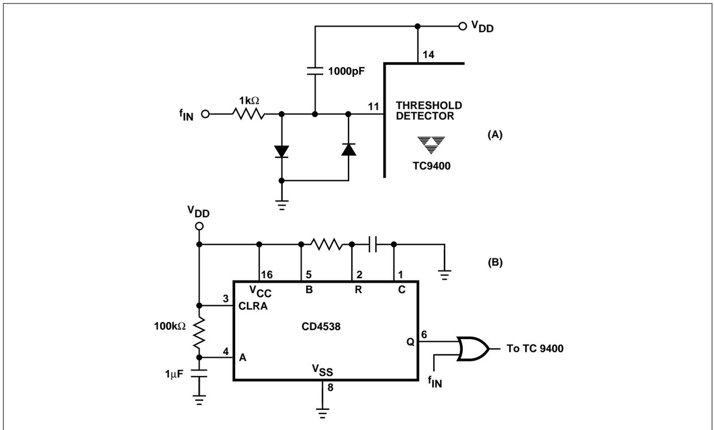
Figure 11. Power-On Operation/Reset
