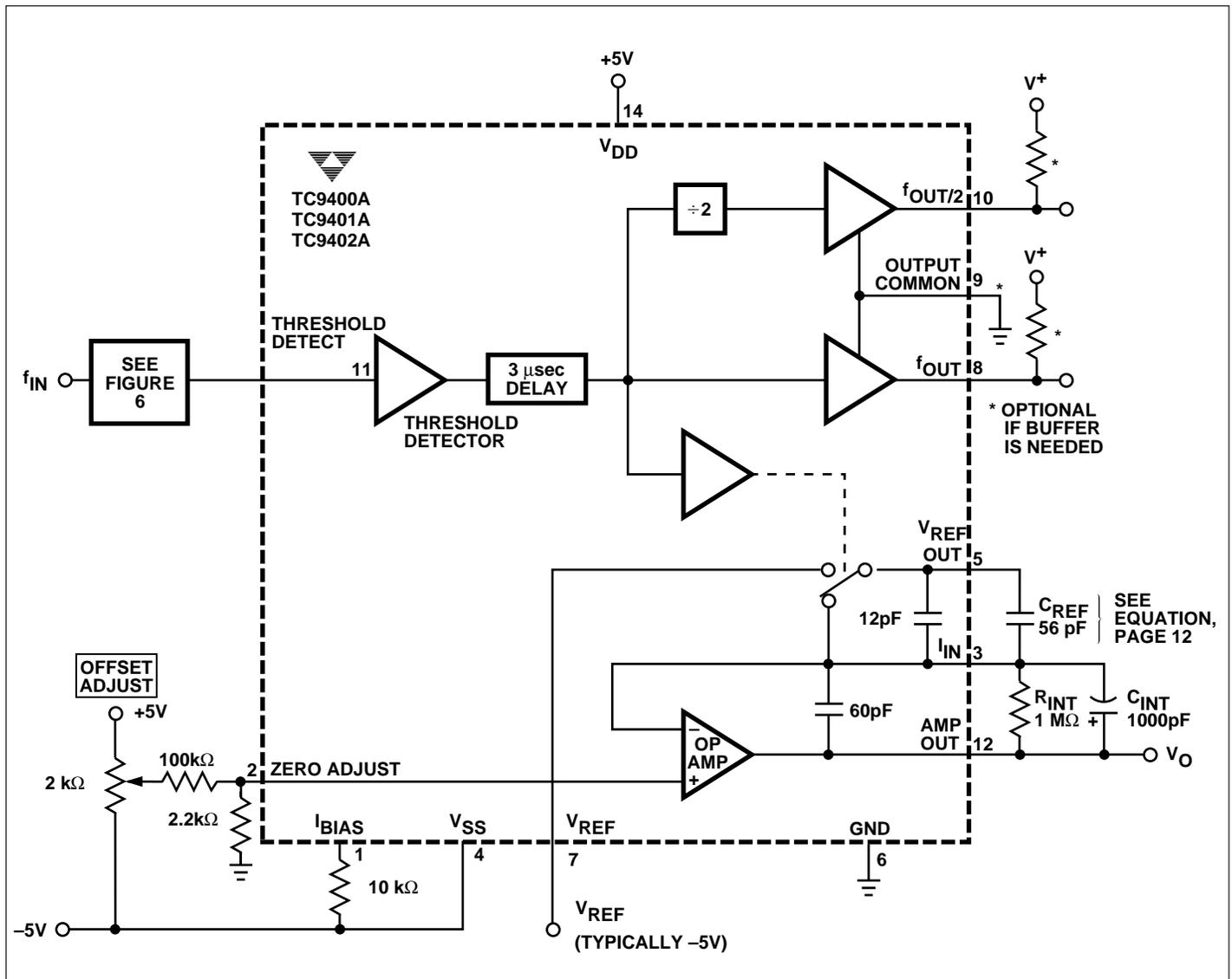
Figure 7. DC — 10 kHz F/V Converter
