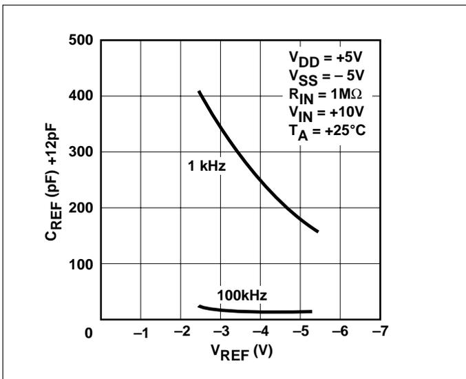
Figure 3. Recommended  $C_{REF}$  VS  $V_{REF}$
