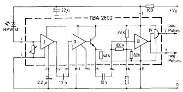
Fig. 1: TBA 2800 block diagram and application circuit
