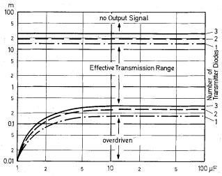
Fig. 3: Transmission range depending on capacitor at pin 2
