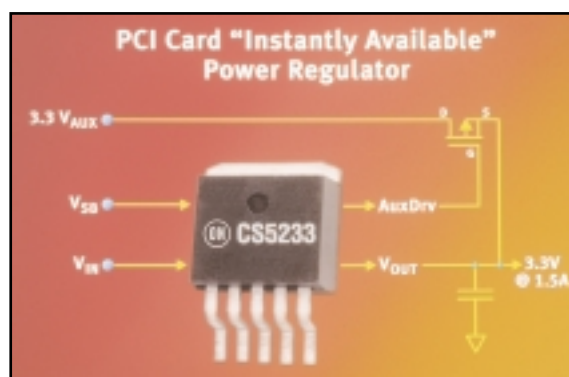
Figure 1. 5V to 3.3V Dual Input Regulator with Auxiliary PFET Power Switch
