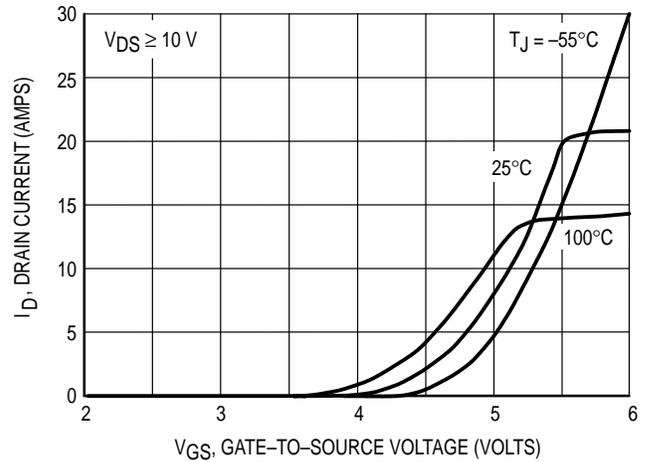
Figure 2. Transfer Characteristics
