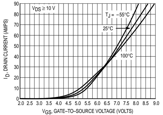
Figure 2. Transfer Characteristics
