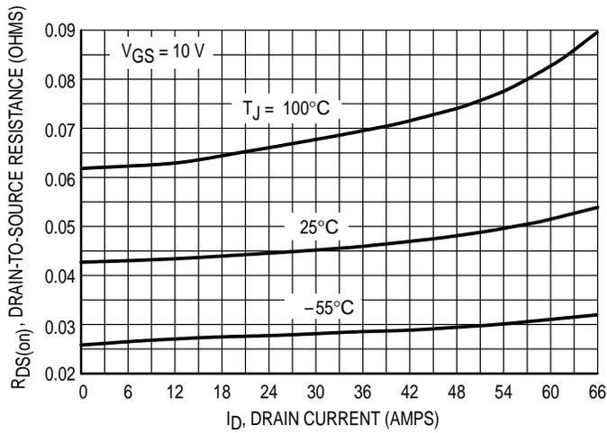
**Figure 3. On-Resistance versus Drain Current and Temperature**
