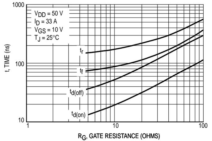
**Figure 9. Resistive Switching Time Variation versus Gate Resistance**
