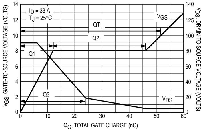
**Figure 8. Gate-To-Source and Drain-To-Source Voltage versus Total Charge**
