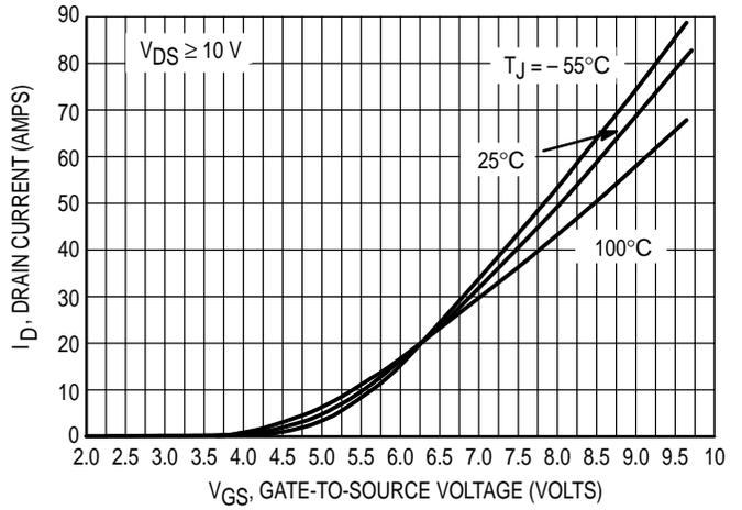
**Figure 2. Transfer Characteristics**
