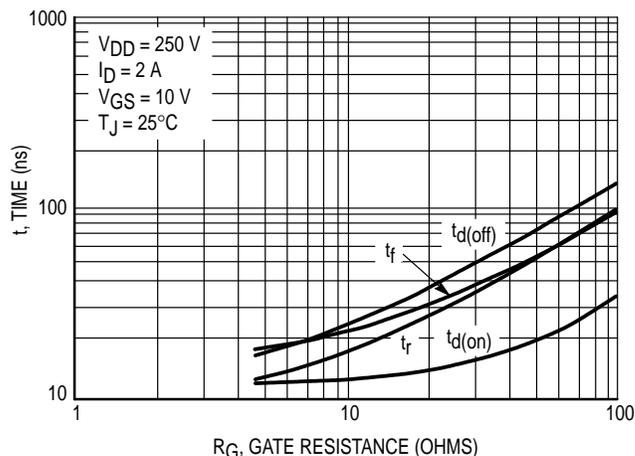
Figure 9. Resistive Switching Time Variation versus Gate Resistance
