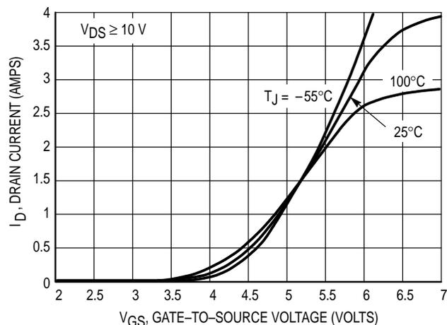
Figure 2. Transfer Characteristics
