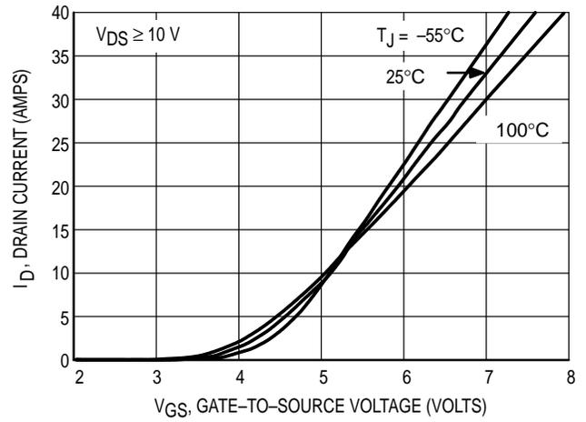
Figure 2. Transfer Characteristics
