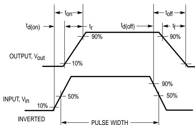
Figure 13. Switching Waveforms
