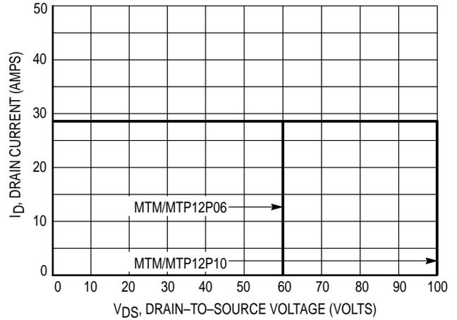
Figure 8. Maximum Rated Switching Safe Operating Area
