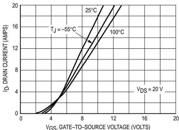
Figure 3. Transfer Characteristics
