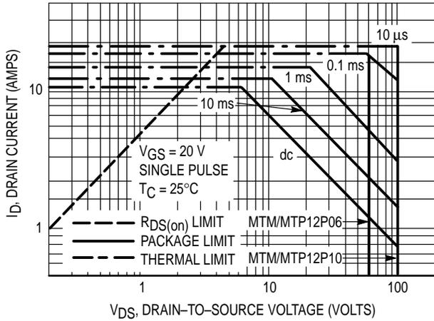
Figure 7. Maximum Rated Forward Biased Safe Operating Area
