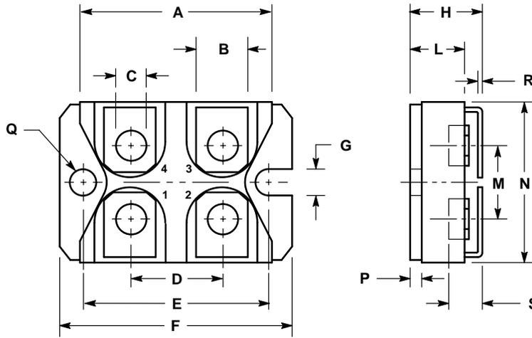
Recommended screw torque:  $1.3 \pm 0.2$  Nm
