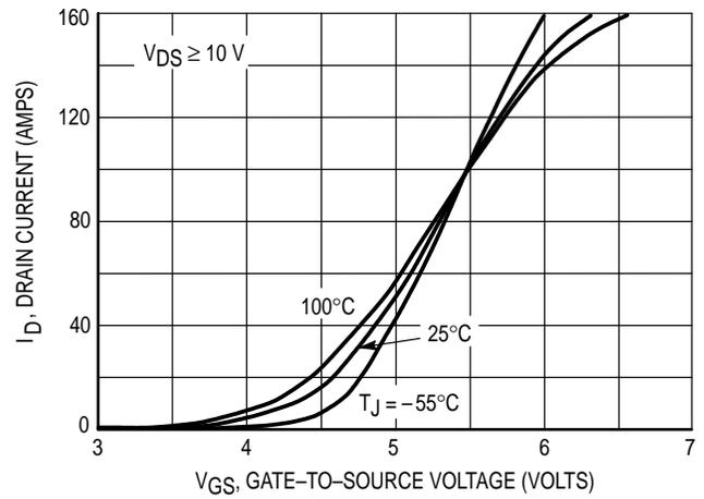
Figure 2. Transfer Characteristics
