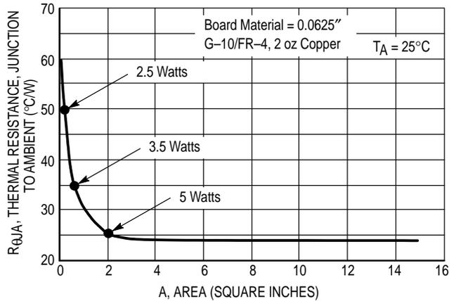
Figure 17. Thermal Resistance versus Drain Pad Area for the D<sup>2</sup>PAK Package (Typical)
