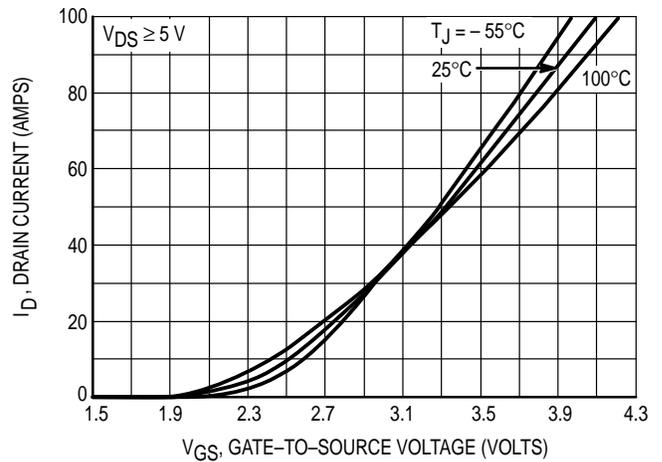
Figure 2. Transfer Characteristics
