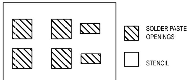
Figure 18. Typical Stencil for DPAK and D<sup>2</sup>PAK Packages
