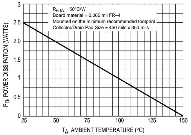
Figure 16. D<sup>2</sup>PAK Power Derating Curve
