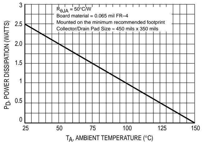
Figure 15. D<sup>2</sup>PAK Power Derating Curve
