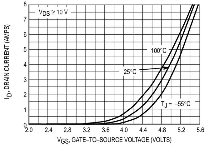
Figure 2. Transfer Characteristics
