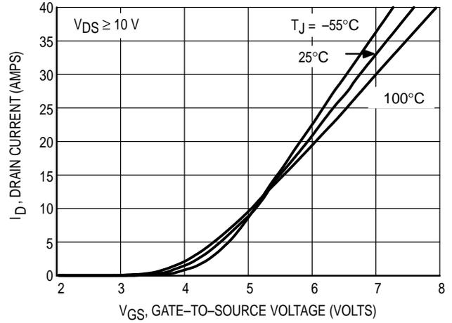
Figure 2. Transfer Characteristics
