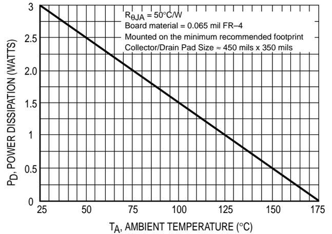
Figure 15. D<sup>2</sup>PAK Power Derating Curve
