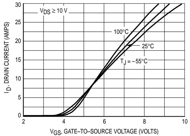
Figure 2. Transfer Characteristics
