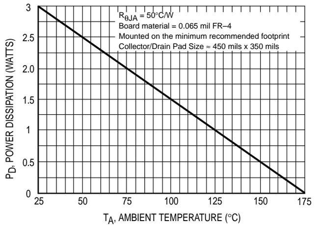
Figure 15. D<sup>2</sup>PAK Power Derating Curve
