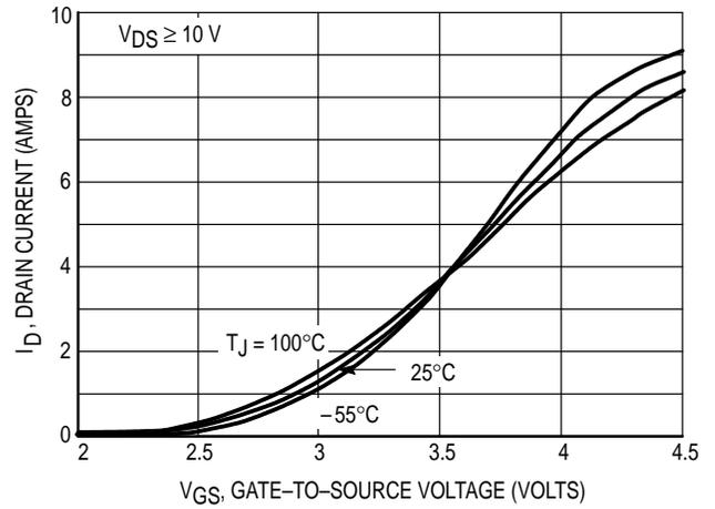
Figure 2. Transfer Characteristics
