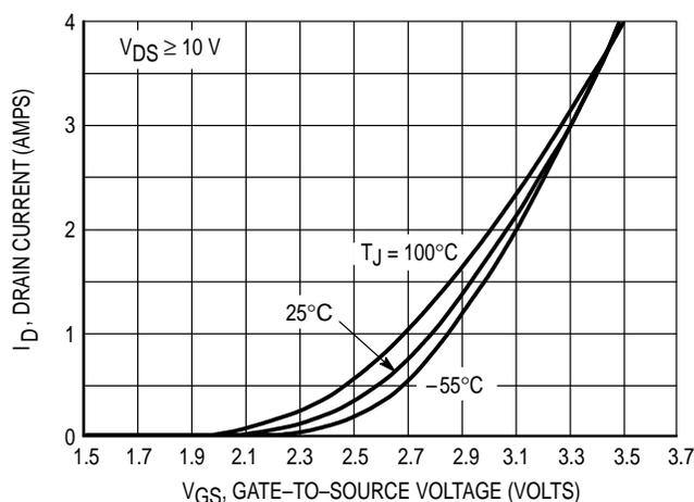
**Figure 2. Transfer Characteristics**
