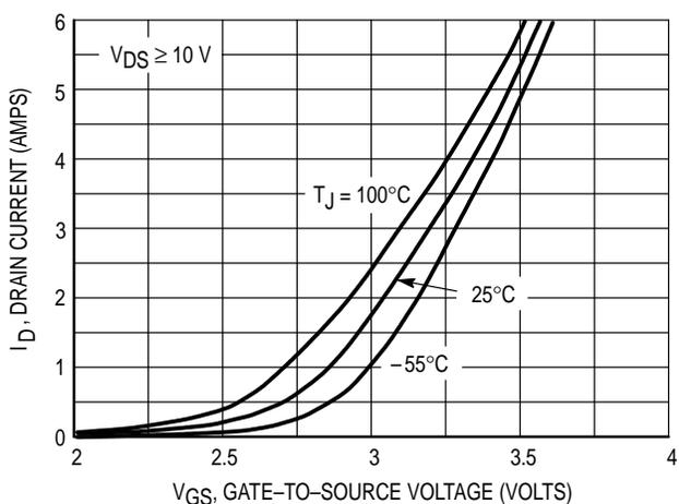
**Figure 2. Transfer Characteristics**
