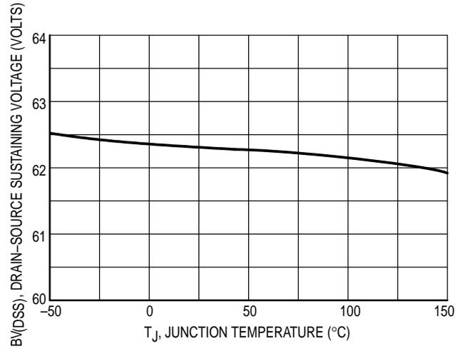
**Figure 7. Drain-Source Sustaining Voltage Variation With Temperature**
