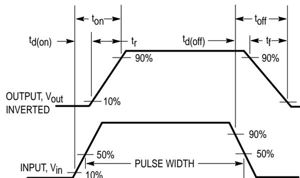
Figure 11. Switching Waveforms
