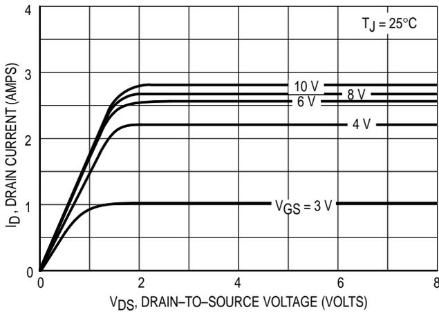
Figure 1. Output Characteristics
