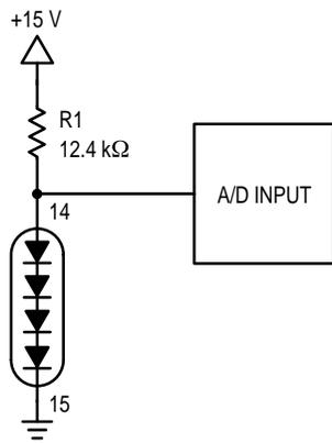
Figure 7. Recommended Temperature Sense Bias Circuit
