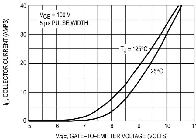
**Figure 3. Transfer Characteristics**
