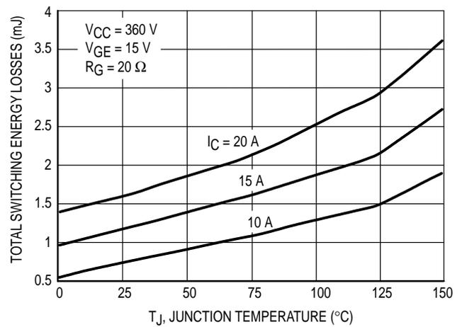
**Figure 8. Total Switching Losses versus Junction Temperature**
