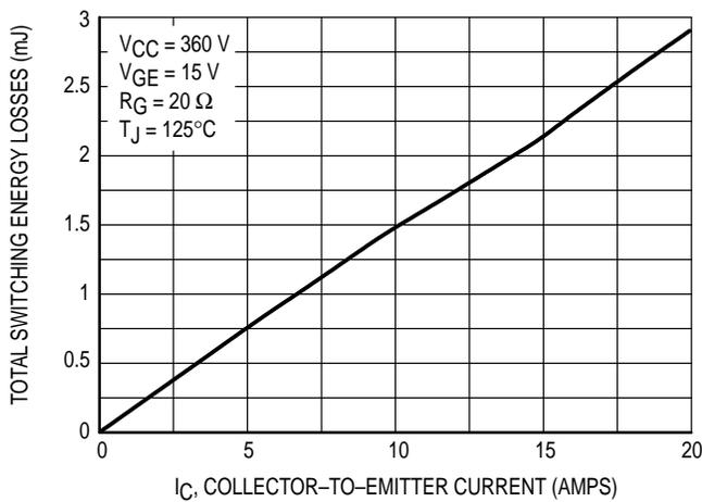
**Figure 9. Total Switching Losses versus Collector-to-Emitter Current**
