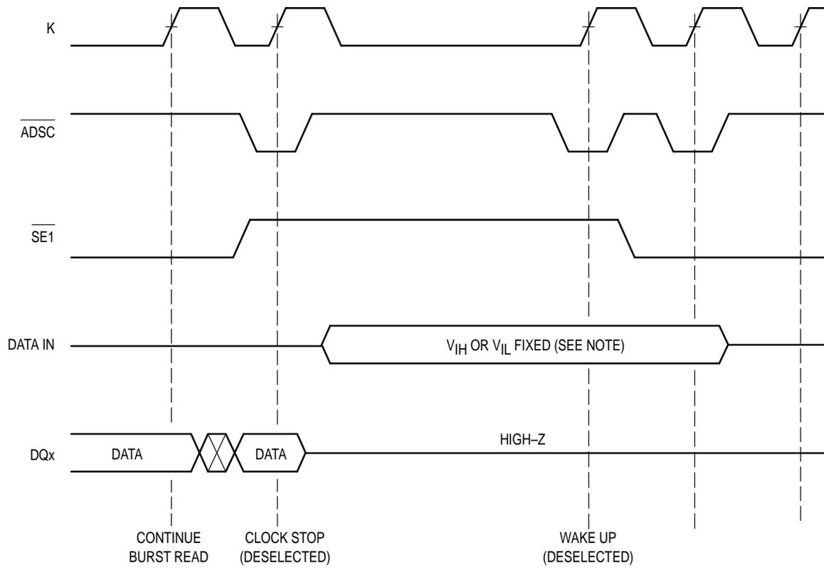
NOTE: While the clock is stopped, DATA IN must be fixed in a high ( $V_{IH}$ ) or low ( $V_{IL}$ ) state to reduce the DC current of the input buffers. For lowest power operation, all data and address lines should be held in a low ( $V_{IL}$ ) state and control lines held in an inactive state.
