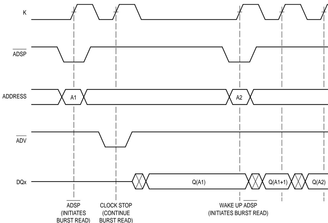
NOTE: For lowest possible power consumption during stop clock, the addresses should be driven to a low state ( $V_{IL}$ ). Best results are obtained if  $V_{IL} < 0.2 V$ .
