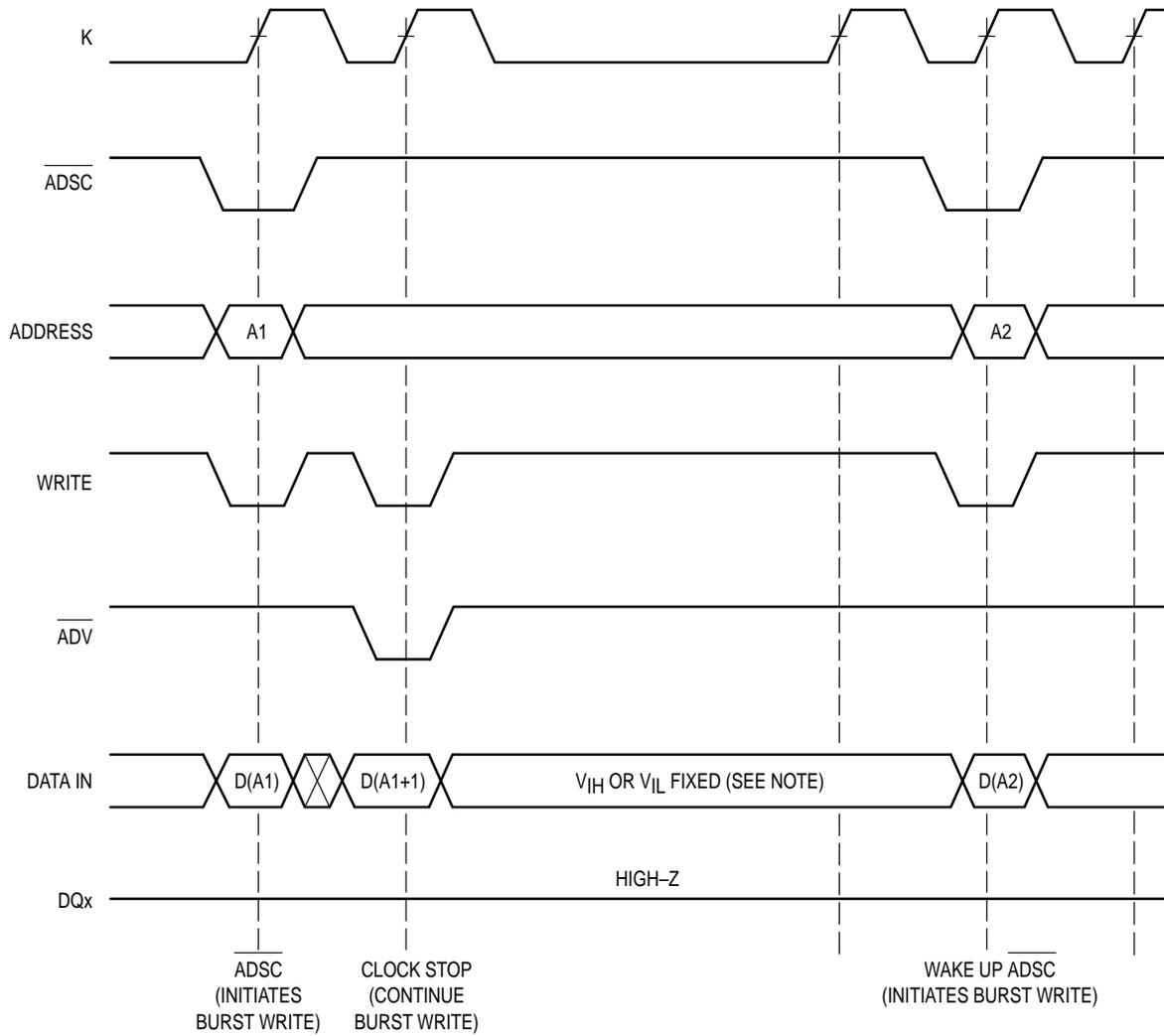
NOTE: While the clock is stopped, DATA IN must be fixed in a high ( $V_{IH}$ ) or low ( $V_{IL}$ ) state to reduce the DC current of the input buffers. For lowest power operation, all data and address lines should be held in a low ( $V_{IL}$ ) state and control lines held in an inactive state.
