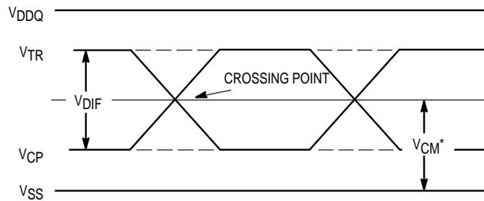
\* $V_{CM}$ , the Common Mode Input Voltage, equals  $V_{TR} - ((V_{TR} - V_{CP})/2)$ .
