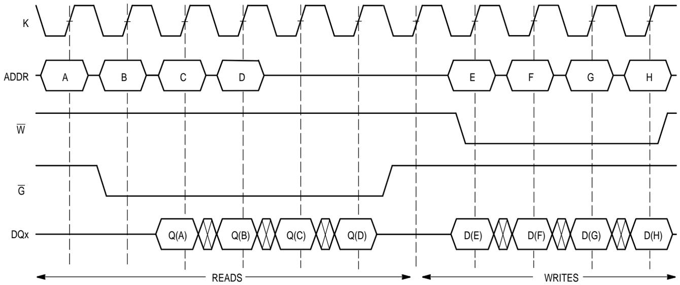
**Figure 2. Configured as Non-Burst Pipelined Synchronous SRAM**
