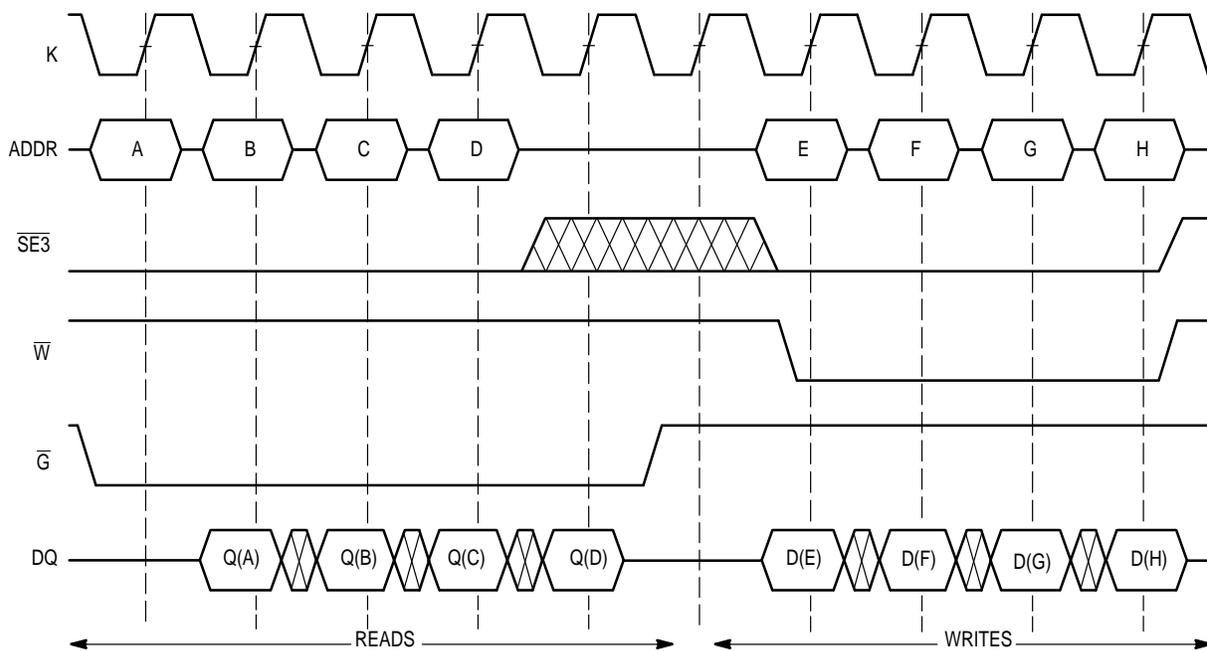
Figure 5. Example Configuration as Non-Burst Synchronous SRAM
