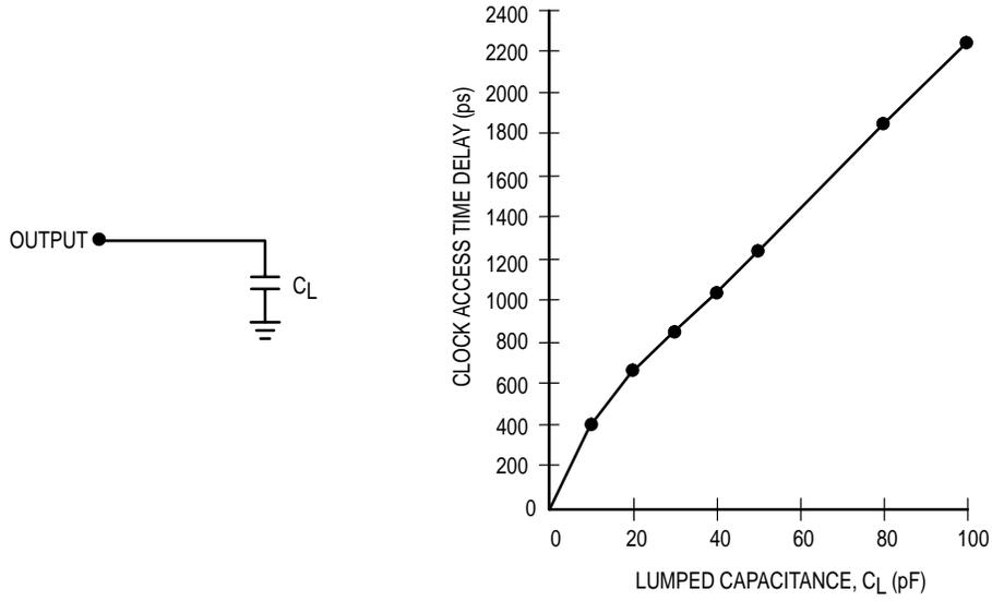
**Figure 3. Lumped Capacitive Load and Typical Derating Curve**
