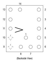
0.116 inch x 0.091 inch Backside orientation marking indicated by arrow oriented as shown
