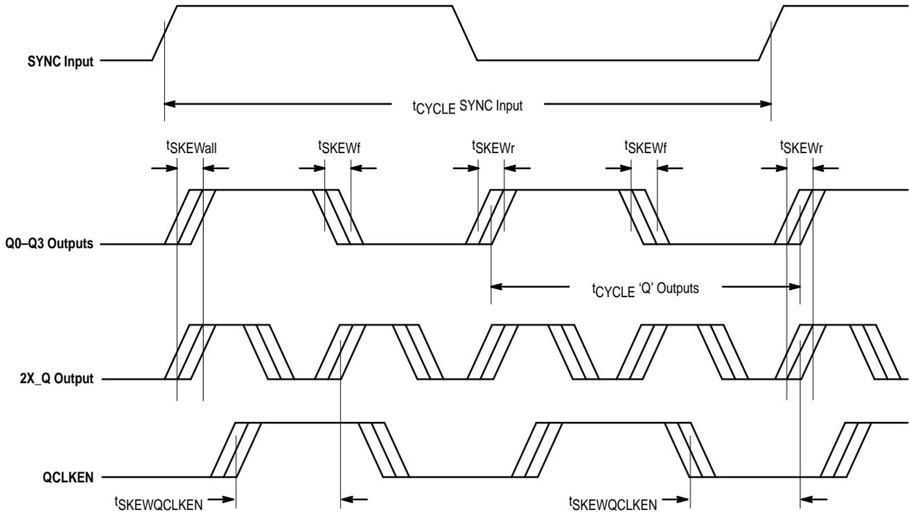
Figure 5. Output/Input Switching Waveforms and Timing Relationships
