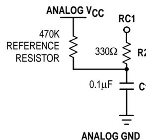
WITH THE 470KΩ RESISTOR TIED IN THIS FASHION THE T<sub>PD</sub> SPECIFICATION, MEASURED AT THE INPUT PINS IS:
