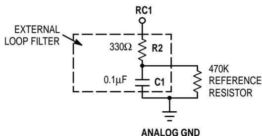
WITH THE 470KΩ RESISTOR TIED IN THIS FASHION THE T<sub>PD</sub> SPECIFICATION, MEASURED AT THE INPUT PINS IS:
