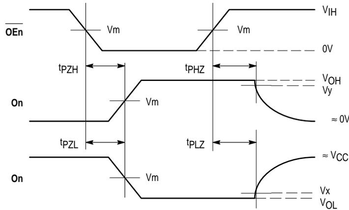
**WAVEFORM 2 - OUTPUT ENABLE AND DISABLE TIMES**
