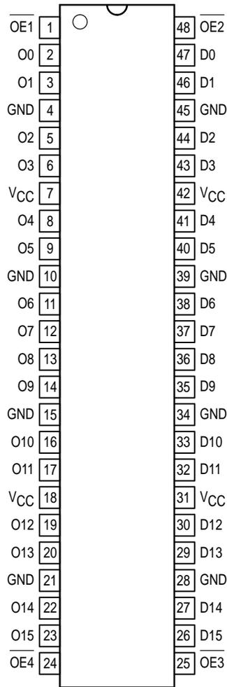
**Figure 1. 48-Lead Pinout**
