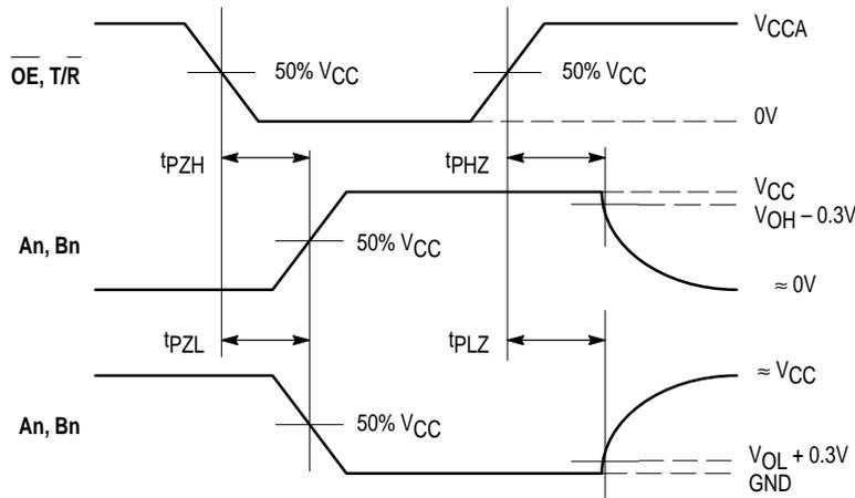
**WAVEFORM 2 – OUTPUT ENABLE AND DISABLE TIMES**
