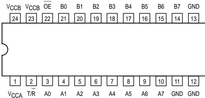
**Figure 1. 24-Lead Pinout**
