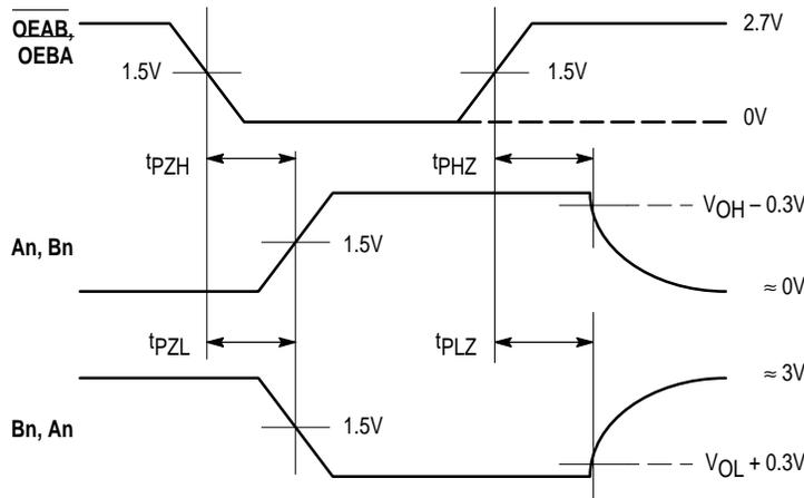
**WAVEFORM 2 – OE<sub>xx</sub> to An/Bn OUTPUT ENABLE AND DISABLE TIMES**
