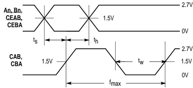
**WAVEFORM 3 – Cxx MINIMUM PULSE WIDTH, An/Bn/CE<sub>xx</sub> to Cxx SETUP AND HOLD TIMES**
