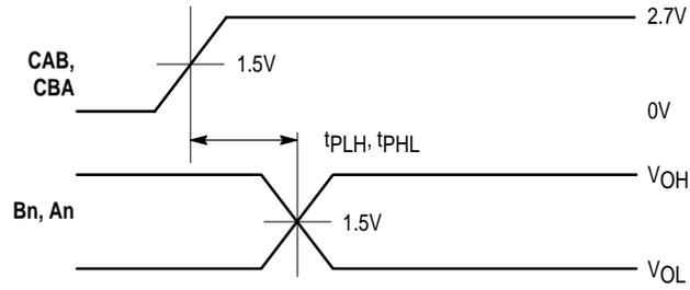
**WAVEFORM 1 – Cxx to An/Bn PROPAGATION DELAYS**
