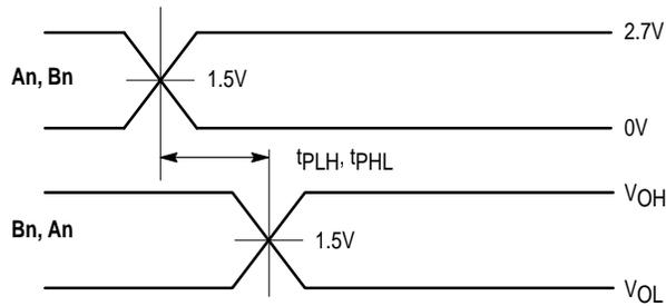
**WAVEFORM 1 – An to Bn PROPAGATION DELAYS**
