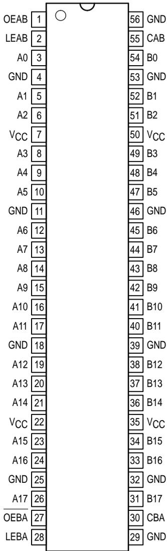
**Figure 1. 56-Lead Pinout
