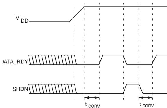
Figure 3. . DATA\_RDY, SHDN Operation Logic Diagram
