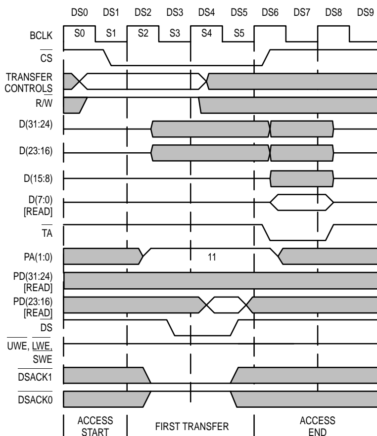
Figure 47. 8-Bit '040 READ From 16-Bit Peripheral Example (PA1,PA0=11)
