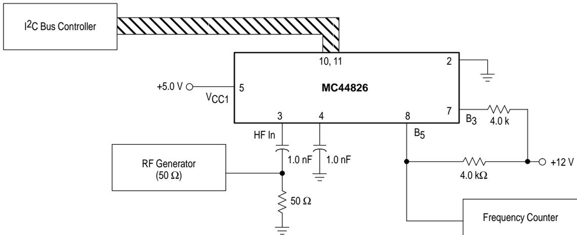
Device is in test mode,  $B_5$  and  $B_3$  are "On",  $B_1$  is "Off".
