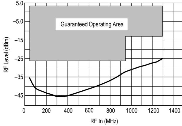
**NOTE:**  $V_{CC} = 4.5$  to  $5.5$  V,  $T_A = -20^\circ$  to  $+80^\circ$  C
