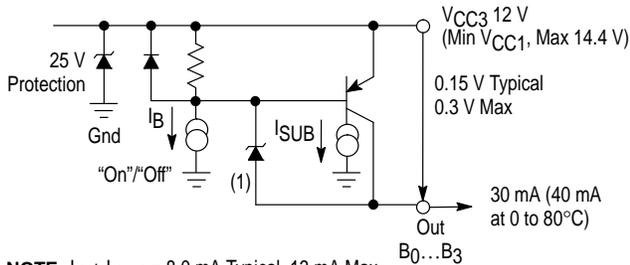
**NOTE:**  $I_B + I_{SUB} = 8.0 \text{ mA Typical, } 13 \text{ mA Max}$
