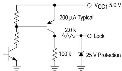
**Figure 6. Typical Tuner Application**
