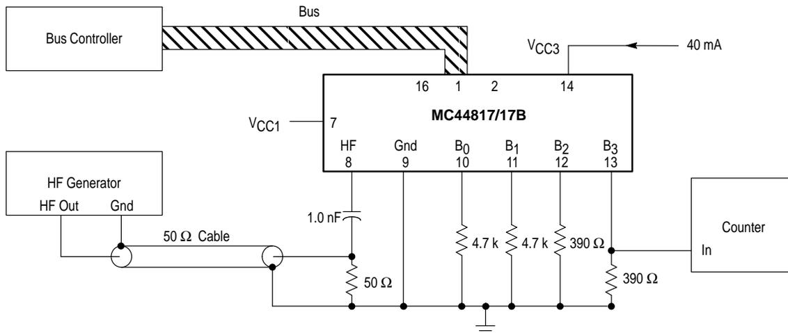
Device is in test mode. B<sub>2</sub>, B<sub>3</sub> are "On" and B<sub>0</sub>, B<sub>1</sub> are "Off".
