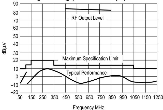
Figure 12. F<sub>O</sub> (Picture Carrier) Harmonics
