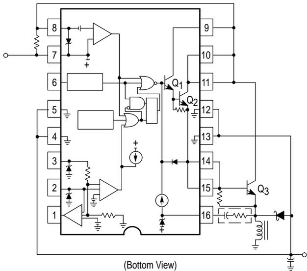
Figure 25B. External PNP Saturated Switch
