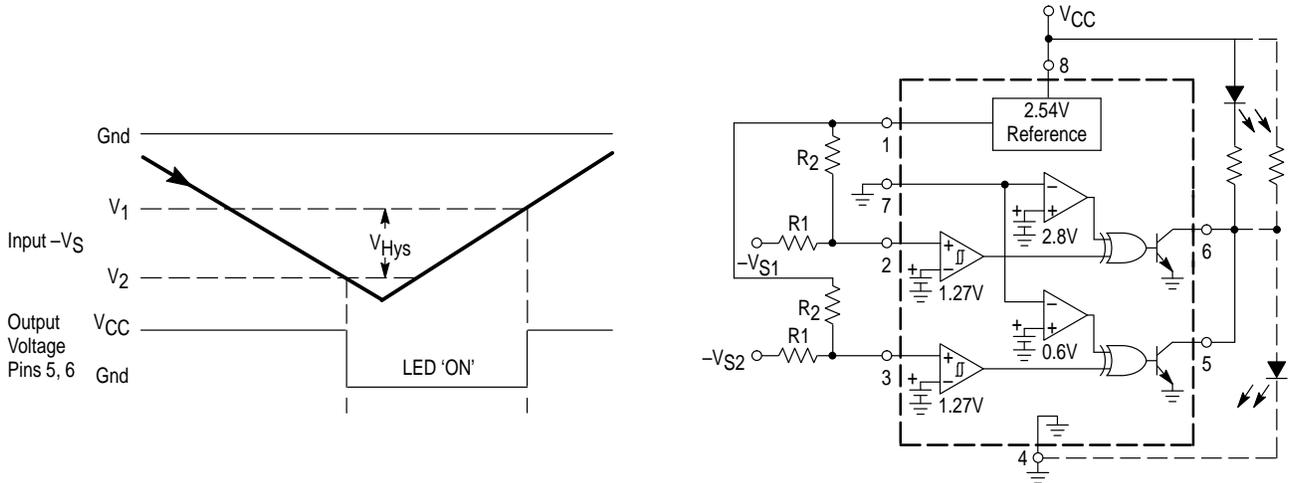
The above figure shows the MC34161 configured as a dual negative overvoltage detector. As the input voltage increases from ground, the LED will turn 'ON' when  $-V_{S1}$  or  $-V_{S2}$  exceeds  $V_2$ . With the dashed line output connection, the circuit becomes a dual negative undervoltage detector. As the input voltage decreases from the peak towards ground, the LED will turn 'ON' when  $-V_{S1}$  or  $-V_{S2}$  falls below  $V_1$ .
