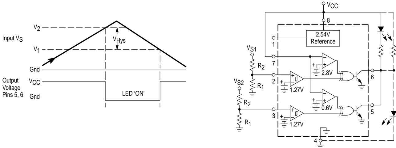
The above figure shows the MC34161 configured as a dual positive overvoltage detector. As the input voltage increases from ground, the LED will turn 'ON' when  $V_{S1}$  or  $V_{S2}$  exceeds  $V_2$ . With the dashed line output connection, the circuit becomes a dual positive undervoltage detector. As the input voltage decreases from the peak towards ground, the LED will turn 'ON' when  $V_{S1}$  or  $V_{S2}$  falls below  $V_1$ .
