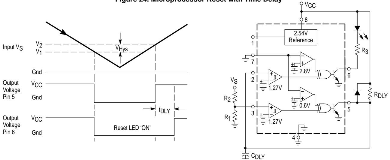
The above figure shows the MC34161 configured as a microprocessor reset with a time delay. Channel 2 monitors input voltage  $V_S$  while channel 1 performs the time delay function. As the input voltage decreases towards ground, the output of channel 2 quickly discharges  $C_{DLY}$  when  $V_S$  falls below  $V_1$ . As the input voltage increases from ground, the output of channel 2 allows  $R_{DLY}$  to charge  $C_{DLY}$  when  $V_S$  exceeds  $V_2$ .
