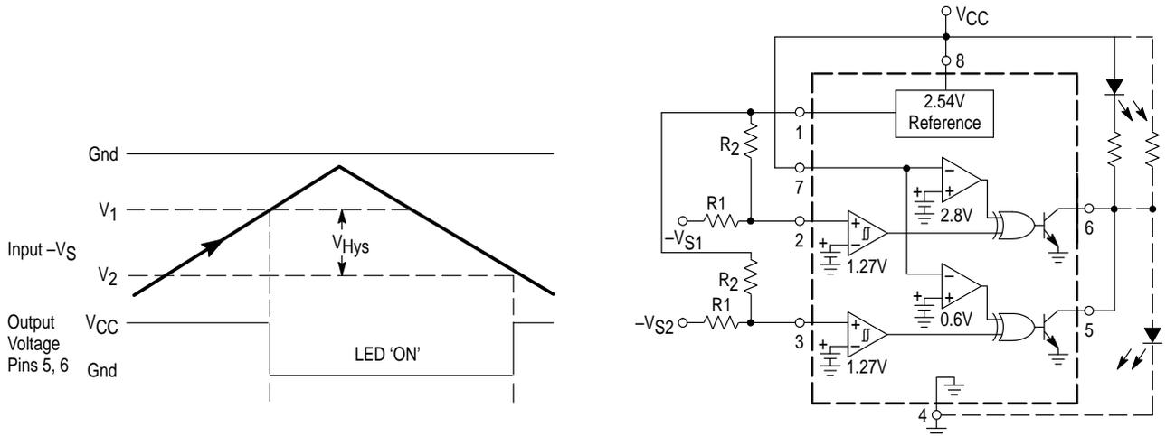
The above figure shows the MC34161 configured as a dual negative undervoltage detector. As the input voltage decreases towards ground, the LED will turn 'ON' when  $-V_{S1}$  or  $-V_{S2}$  falls below  $V_1$ . With the dashed line output connection, the circuit becomes a dual negative overvoltage detector. As the input voltage increases from ground, the LED will turn 'ON' when  $-V_{S1}$  or  $-V_{S2}$  exceeds  $V_2$ .
