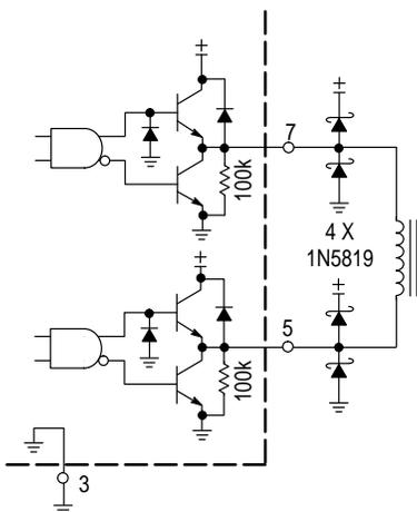
Output Schottky diodes are recommended when driving inductive loads at high frequencies. The diodes reduce the driver's power dissipation by preventing the output pins from being driven above  $V_{CC}$  and below ground.
