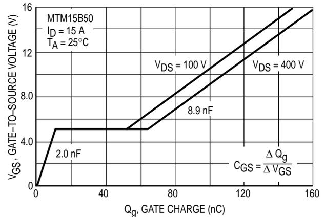
The capacitive load power dissipation is directly related to the required gate charge, and operating frequency. The capacitive load power dissipation per driver is:
