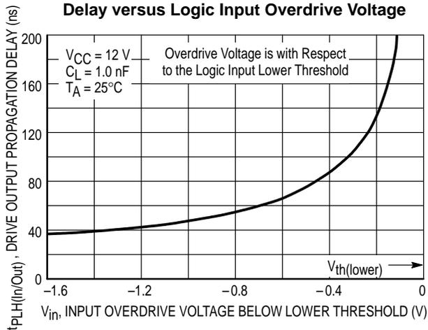
Figure 6. Drive Output Low to High Propagation Delay versus Logic Input Overdrive Voltage
