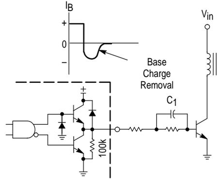
The totem-pole outputs can furnish negative base current for enhanced transistor turn-off, with the addition of capacitor C<sub>1</sub>.
