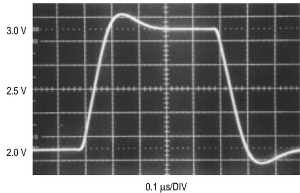
Figure 7. Reference Voltage Change versus Source Current
