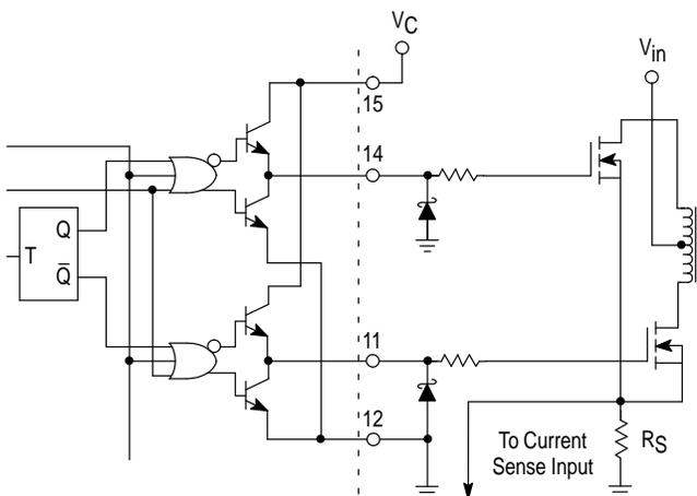
A series gate resistor may be needed to damp high frequency parasitic oscillation caused by a MOSFET's input capacitance and any series wiring inductance in the gate-source circuit. The series resistor will also decrease the MOSFET's switching speed. A Schottky diode can reduce the driver's power dissipation due to excessive ringing, by preventing the output pin from being driven below ground. The Schottky diode also prevents substrate injection when the output pin is driven below ground.
