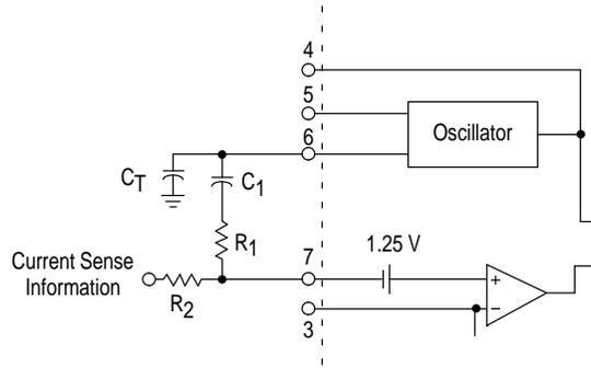
This method of slope compensation is easy to implement, however, it is noise sensitive. Capacitor  $C_1$  provides AC coupling. The oscillator signal is added to the current signal by a voltage divider consisting of resistors  $R_1$  and  $R_2$ .
