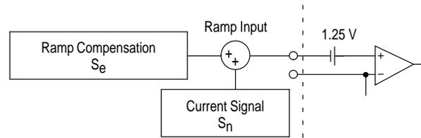
A simple equation can be used to calculate the amount of external ramp necessary to add that will achieve stability in the current loop. For the following equations, the calculated values for the application circuit in Figure 36 are also shown.
