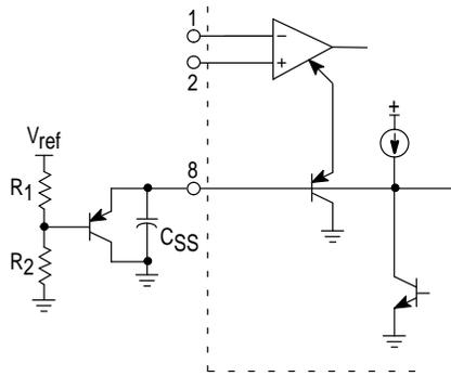
In voltage mode operation, the maximum duty cycle can be clamped. By the addition of a PNP transistor to buffer the clamp voltage, the Soft-Start current is not affected by R<sub>1</sub>.
