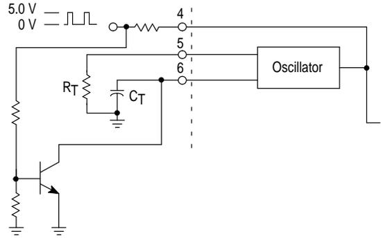
The sync pulse fed into the clock pin must be at least 3.9 V.  $R_T$  and  $C_T$  need to be set 10% slower than the sync frequency. This circuit is also used in voltage mode operation for master/slave operation. The clock signal would be coming from the master which is set at the desired operating frequency, while the slave is set 10% slower.
