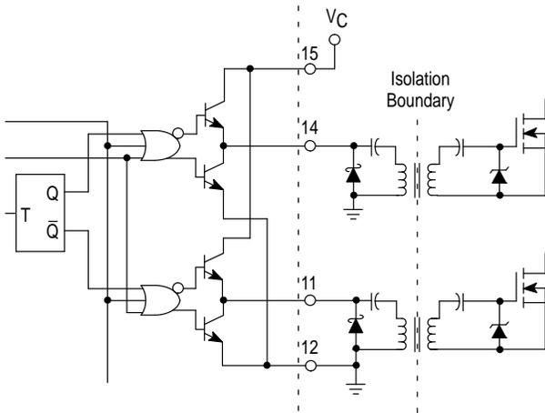
The totem pole output can easily drive pulse transformers. A Schottky diode is recommended when driving inductive loads at high frequencies. The diode can reduce the driver's power dissipation due to excessive ringing, by preventing the output pin from being driven below ground.
