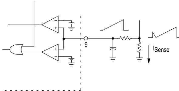
The addition of an RC filter will eliminate instability caused by the leading edge spike on the current waveform. This sense signal can also be used at the ramp input pin for current mode control. For ramp compensation it is necessary to know the gain of the current feedback loop. If a transformer is used, the gain can be calculated by:
