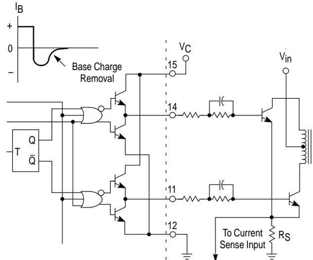
The totem pole output can furnish negative base current for enhanced transistor turn-off, with the addition of the capacitor in series with the base.
