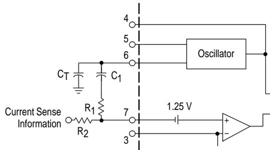
This method of slope compensation is easy to implement, however, it is noise sensitive. Capacitor  $C_1$  provides AC coupling. The oscillator signal is added to the current signal by a voltage divider consisting of resistors  $R_1$  and  $R_2$ .
