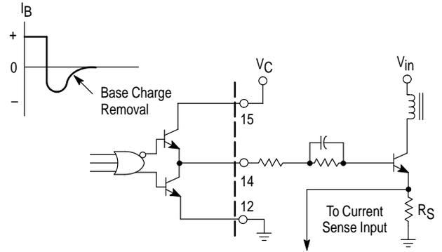
The totem pole output can furnish negative base current for enhanced transistor turn-off, with the addition of the capacitor in series with the base.
