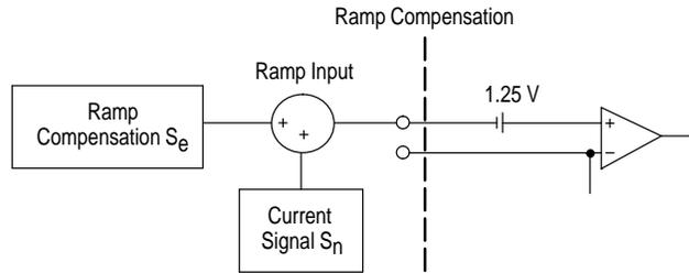
A simple equation can be used to calculate the amount of external ramp slope necessary to add that will achieve stability in the current loop. For the following equations, the calculated values for the application circuit in Figure 34 are also shown.
