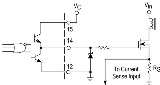
A series gate resistor may be needed to dampen high frequency parasitic oscillation caused by the MOSFET's input capacitance and any series wiring inductance in the gate-source circuit. The series resistor will also decrease the MOSFET switching speed. A Schottky diode can reduce the driver's power dissipation due to excessive ringing, by preventing the output pin from being driven below ground. The Schottky diode also prevents substrate injection when the output pin is driven below ground.
