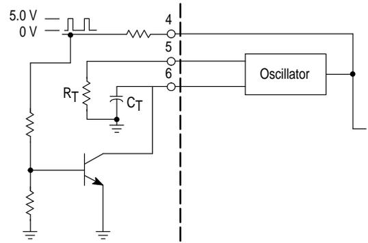
The sync pulse fed into the clock pin must be at least 3.9 V.  $R_T$  and  $C_T$  need to be set 10% slower than the sync frequency. This circuit is also used in Voltage Mode operation for master/slave operation. The clock signal would be coming from the master which is set at the desired operating frequency, while the slave is set 10% slower.
