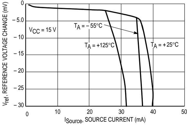
Figure 8. Reference Short Circuit Current versus Temperature
