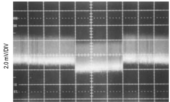
$V_{ref}$  LOAD REGULATION 1.0 mA to 10 mA
