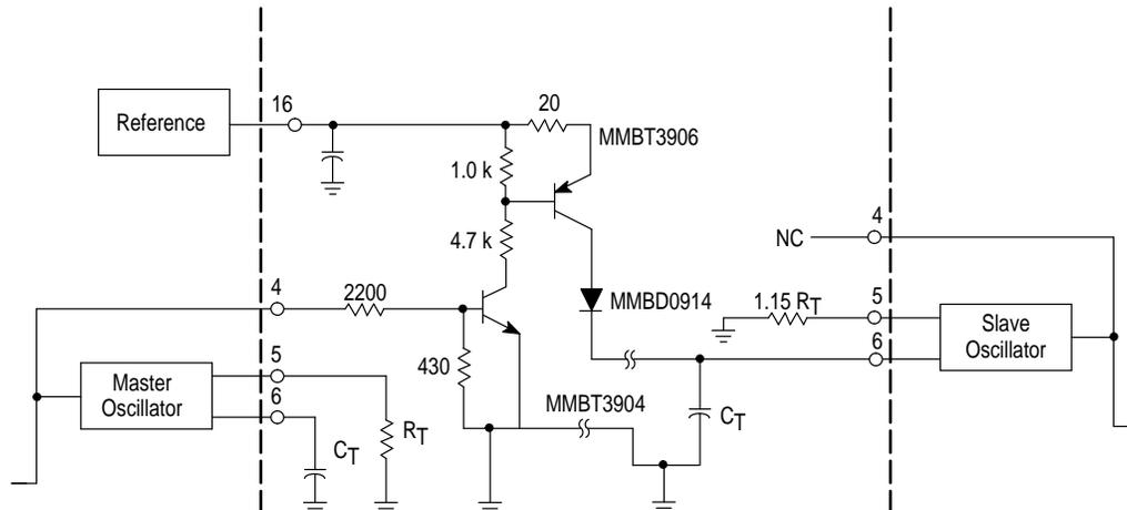
Figure 30. Buffered Maximum Clamp Level
