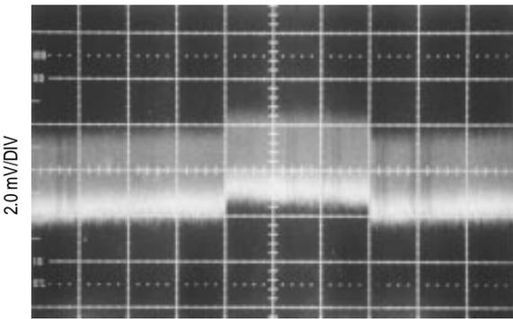
$V_{ref}$  LINE REGULATION 10 V to 24 V
