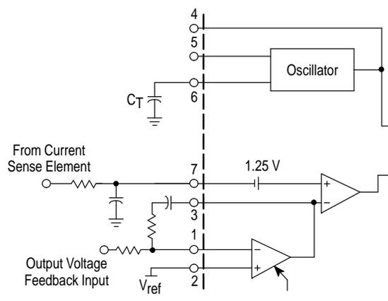
In current mode control, an RC filter should be placed at the ramp input to filter the leading edge spike caused by turn-on of a power MOSFET.
