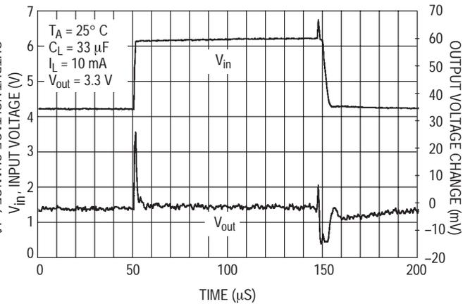
Figure 3. Load Transient Response
