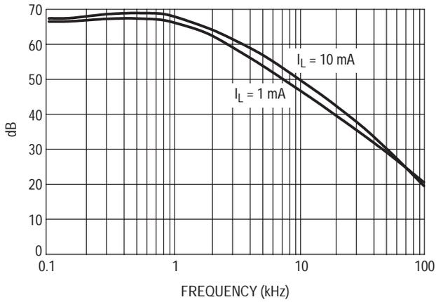
Figure 13. Ripple Rejection
