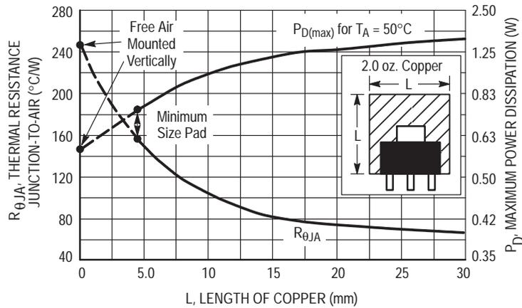
**Figure 25. SOP-8 Thermal Resistance and Maximum Power Dissipation versus P.C.B. Copper Length**
