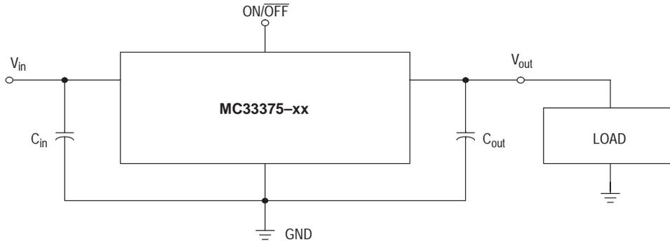
The MC33375 regulators are designed with internal current limiting and thermal shutdown making them user-friendly. Figure 15 is a typical application circuit. The output capability of the regulator is in excess of 300 mA, with a typical dropout voltage of less than 260 mV. Internal protective features include current and thermal limiting.
