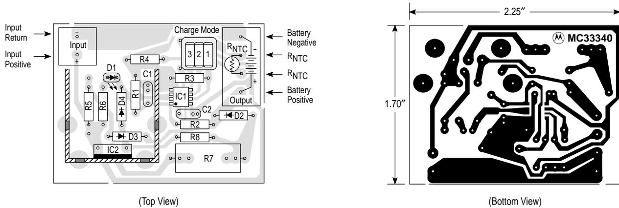
**Figure 15. Line Isolated Switch Mode Charger**
