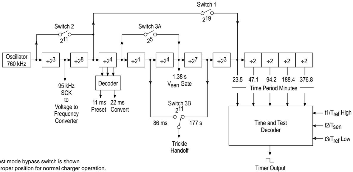
Each test mode bypass switch is shown in the proper position for normal charger operation.
